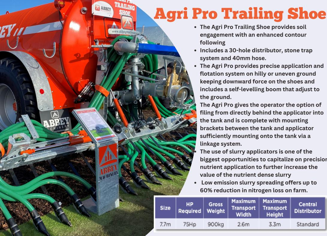
• The Agri Pro Trailing Shoe provides soil engagement with an enhanced contour following
